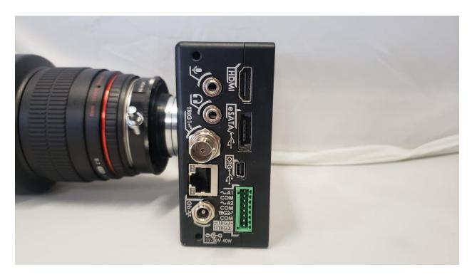
2. Plug the end of the trigger cable into the BNC port. It will press in and twist to the right. Note that when using a BNC trigger, if the cable isn't long enough, you can use a BNC extension cable. Krontech sells up to 90 feet extensions with the ability to stack multiple to increase the length further, or chain multiple cameras to one trigger.
