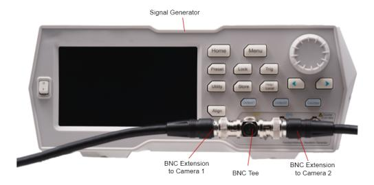
• Connect a BNC Extension Cable to the I/O1 BNC port of each camera. This type of connection is more common with signal generators.
