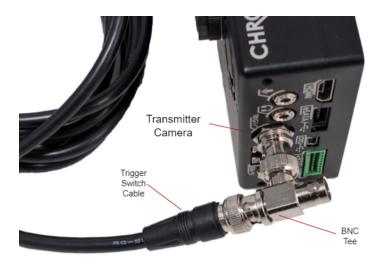
• Connect the receiver BNC extension cable to the BNC Tee on the transmitter camera.
