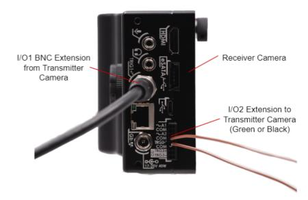
• The final camera setup should appear to be similar to the diagram shown below.
