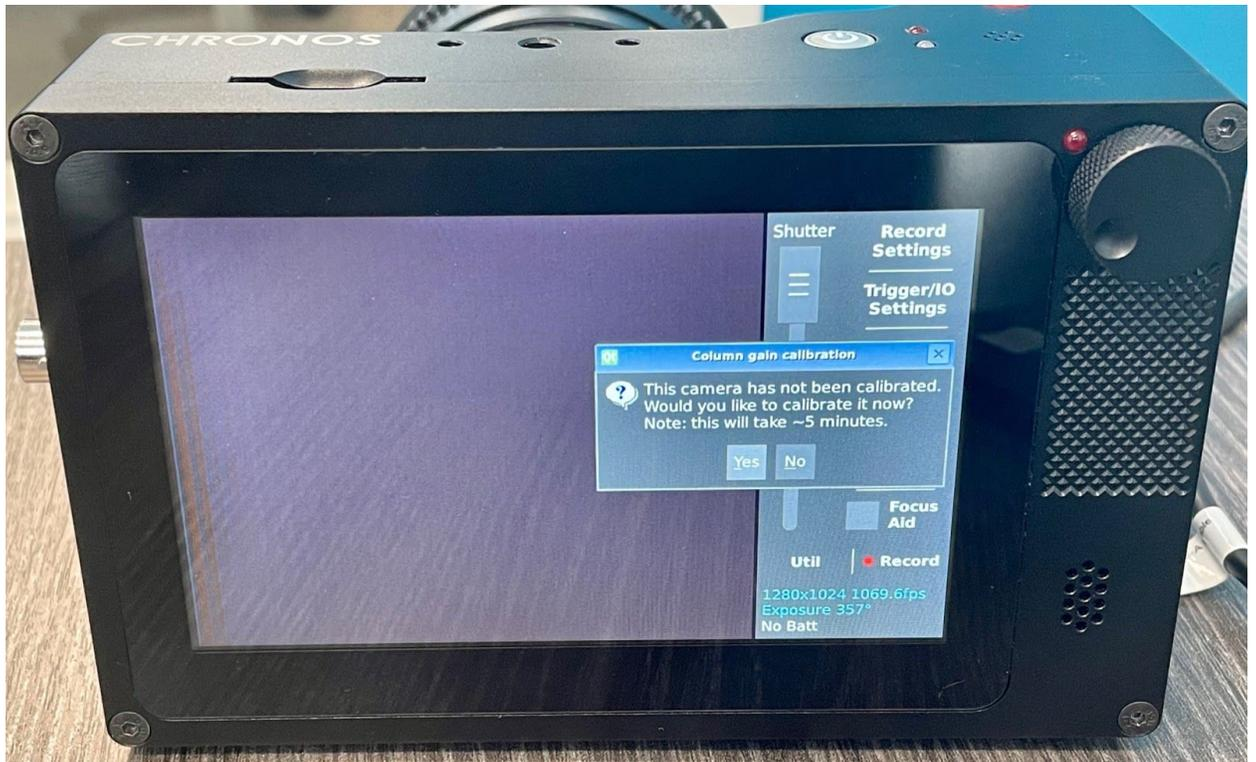
Wait for 15 minutes to let the camera and image sensor reach their operating temperatures, then press **Yes**. This procedure can be redone at any time via the Util -> Factory screen.
