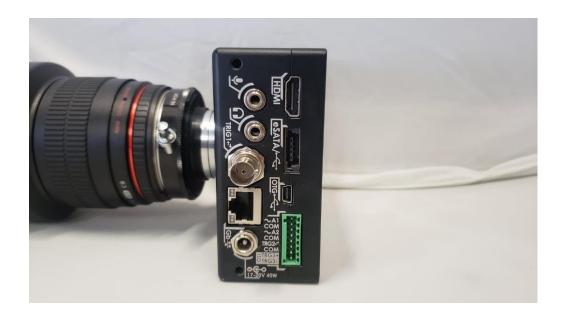
2. Plug the end of the trigger cable into the BNC port. It will press in and twist to the right. Note that when using a BNC trigger and the cable isn't long enough, you can use a BNC extension cable. Krontech sells up to 90 feet extensions with the ability to daisy chain multiple to increase the length further, or chain multiple cameras to one trigger. See www.krontech.ca/store
