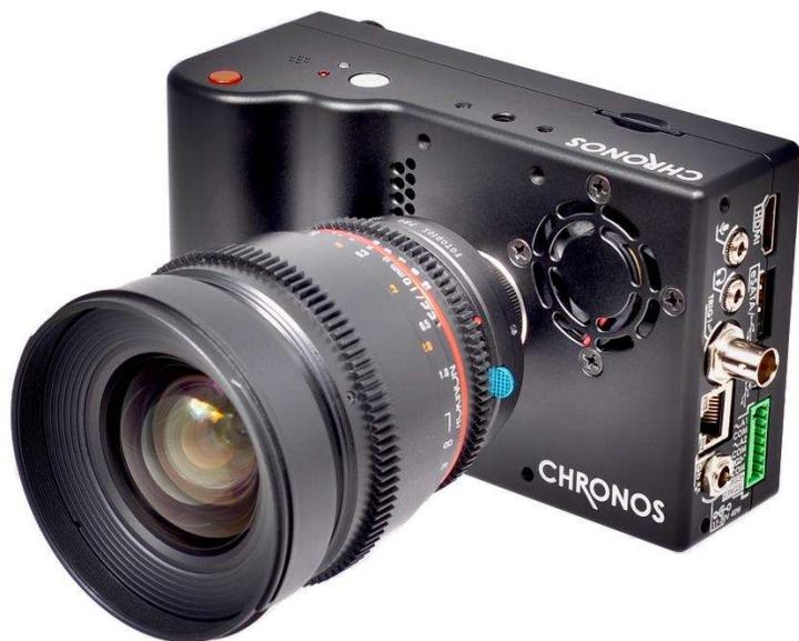
Chronos 2.1-HD is a 1080p1000, 2.1 gigapixel-per-second handheld high-speed camera. Completely self-contained, you can take high-speed imaging with you anywhere! It records 1080p video at 1000fps, and can record at up to 100 000fps at lower resolutions. Video is saved to removable media in compressed h.264 or uncompressed dng format. You can shoot for hours, saving hundreds of shots on a single card.
